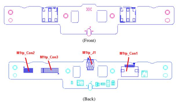
Figure B-4 Touchpad Board layout (front/back)
